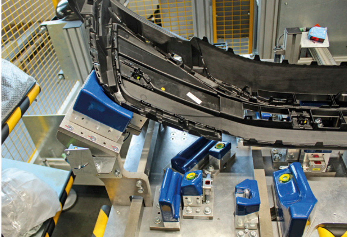
Painted car bumpers are placed in this LASE assembly cell to punch ultrasonic holes for parking sensors
