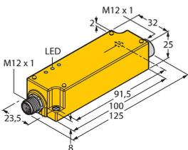
2-channel isolating switching amplifier with M12x1 males, for peripheral use, IP67, zones 2/22, input circuits II(1) Ex ia, PNP transistor output NO
