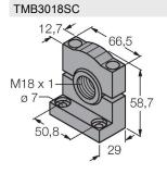
7700397 Mounting bracket, PBT black, for 18 mm thread
