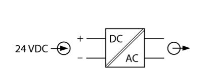
The PSM24... power supply module supplies the excom system with power to the full extension. The power supply module can be used in Zone 2.
