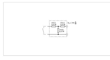
The resistor module meets the requirements of line monitoring between a mechanical contact and a TURCK signal processor. The input circuit of the signal processor is designed for sensors acc. to EN60947-5-6 (NAMUR) and equipped with a wire-break and short-circuit monitoring function.
