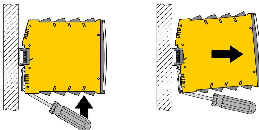
Fig. 4: Remove device
