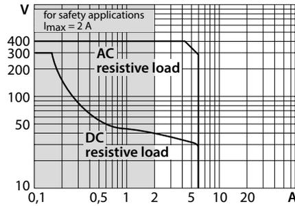
Fig. 5: Load Curve
