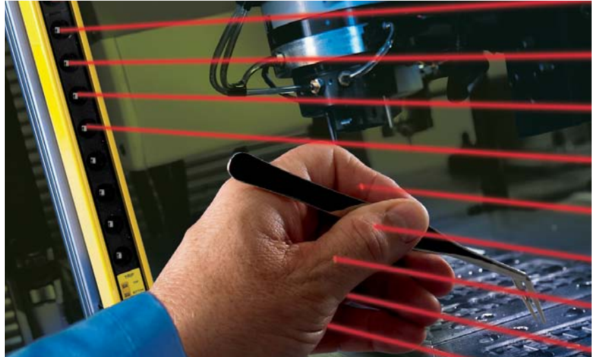
Safety Light Screen Q32L – light screen triggers start and stop of machine
