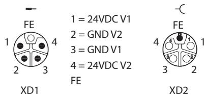
Fig. 8: Pin assignment voltage supply connectors, M12, 5-pin
