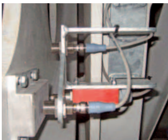
Two uprox+ sensors record a special cam to reliably determine the current position of the blade angle
